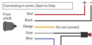
MOB+ can be installed together with your existing kill switch by connecting it in series or parallel. If you should connect in series or parallel depends on your existing kill switch function. The above picture shows an example with Normally Closed connection.
